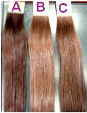
Fig. 3: Color wash fastness efficiency of ABIL® ME 45 – Differences in color after 20 washing cycles
