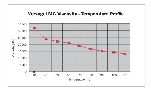
Like the other Versagel products, Versagel MC is shear thinning. However, the Versagel MC products are unique in that they exhibit minimal "stringiness" due to the short hydrocarbon chain structure of the base oil. This characteristic is desirable in certain applications where elasticity needs to be minimized. The graph shows a how viscosity decreases as the temperature decreases for Versagel MC 750.
