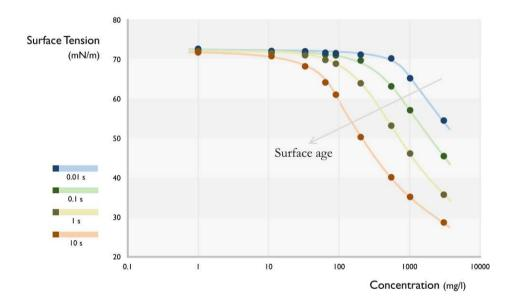
Fig. 3 Dynamic surface tension vs. concentration for SYNETH™ C15 measured at different surface ages. Measurement were conducted at room temperature (25.0 ± 0.1°C) using a KRUSS BP100 Bubble Pressure Tensiometer.
