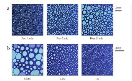
Fig 5 a) Evolution of foam structure for 5% SYNETH™ C15 in water; b) Foam structure of aqueous solutions of SYNETH™ C15 at different concentrations 20 seconds after sparging was completed. Images were obtained using a KRUSS DFA100 Dynamic Foam Analyzer with a Foam Structure Analyzer Module. Foam was generated by sparging air into the solution at 0.2 l/min for 10 seconds. Measurements were carried out at room temperature (25.0 ± 0.1°C). Scale is 2mm.
